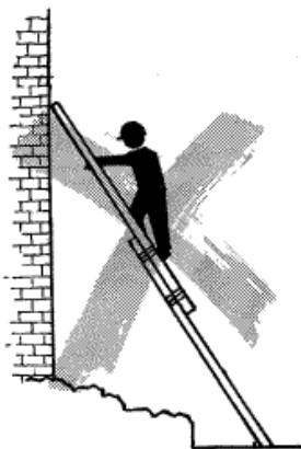
Instability - Base of ladder positioned too far from wall. Sudden slipping can occur.
