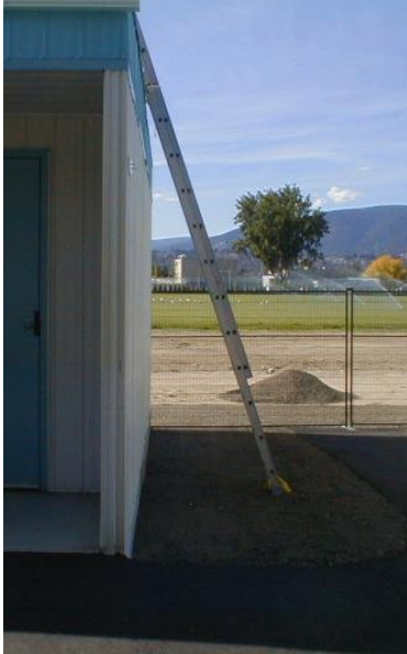
Proper 4 to 1 set-up outside a portable
